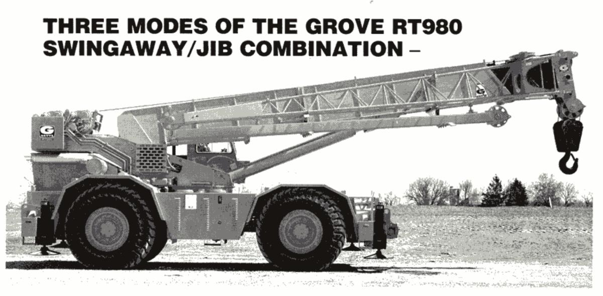
The 32 ft. Swingaway and optional 28 ft. A-frame jib can provide the RT980 with an additional 60 ft. of reach capability, conveniently stowed on the crane. The three different modes of this combination are:
